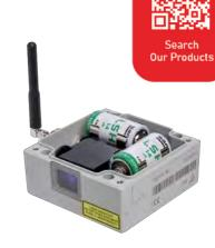
The LaserTilt90 wireless sensor is a 2-in-1 laser distance meter and tiltmeter. The laser measures the relative distance between pairs of reference points. One of the two points can be a natural surface or target foils while the node can be placed at the other end point. Meanwhile, the tiltmeter provides measurements of changes from the vertical level, either on the ground or in structures and is used to monitor inclinations, movements and differential settlements of slopes or infrastructures.
