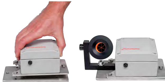
The Tilt90-i mounted on a double plate for horizontal surface mounting (LS-ACC-IN15DP). This is suitable for applications that need to eliminate the need to open the casing during installation. The plate includes a threaded hole available for installing a monitoring prism or a button head screw for precise levelling.
